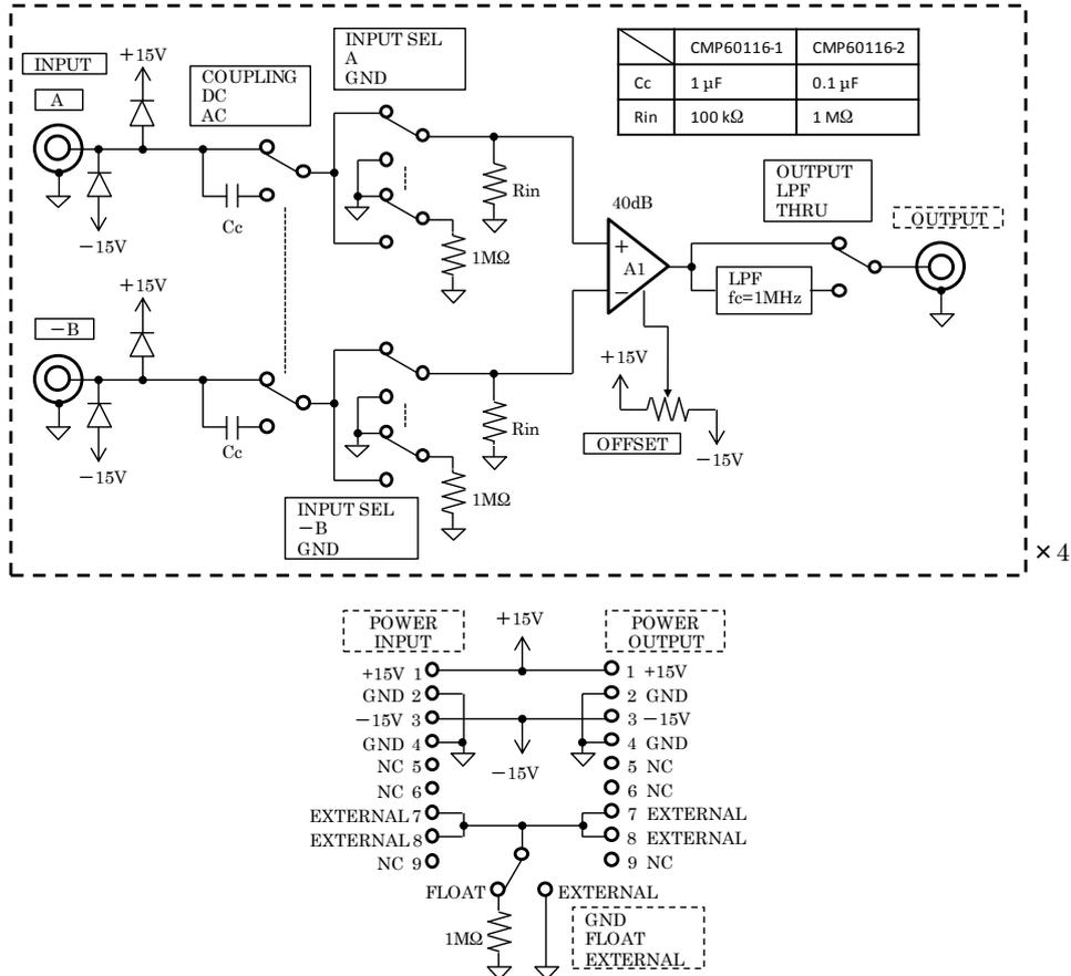
Figure 1-1 Block diagram.
