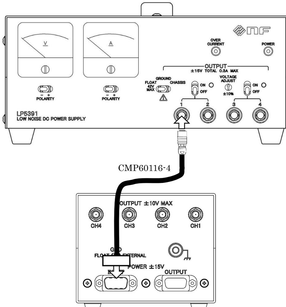
Figure 2-1 Connecting to LP5391.
