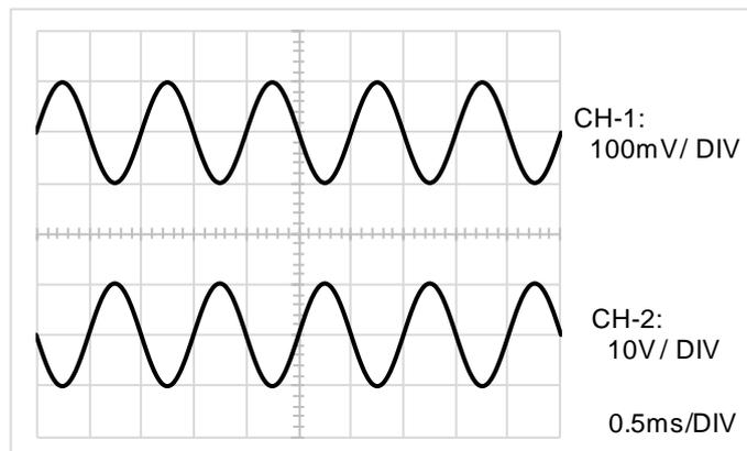
Figure 4-4 Inverting input / output voltage waveform.
