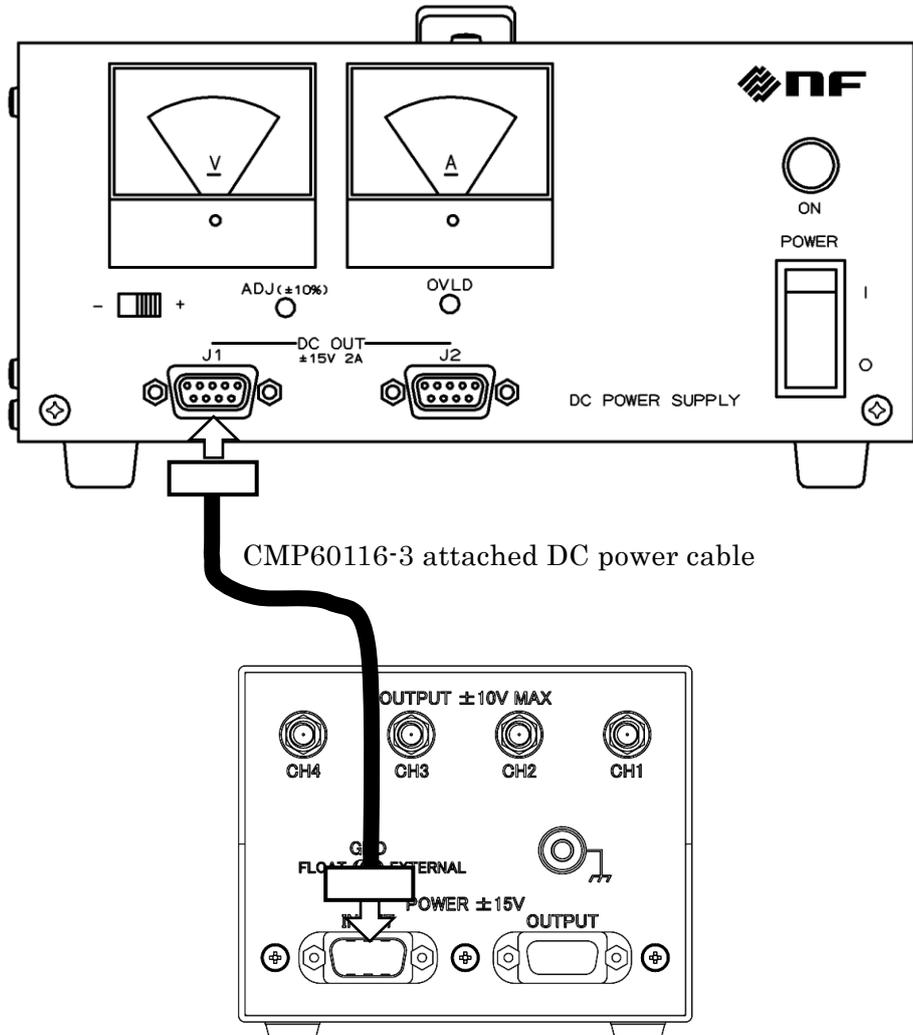
Figure 2-2 Connecting to CMP60116-3.
