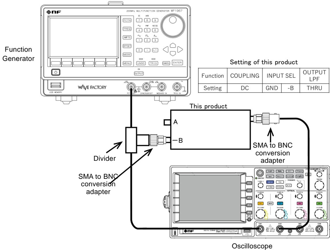
Figure 4-3 Connection diagram for checking inverting input operation.
