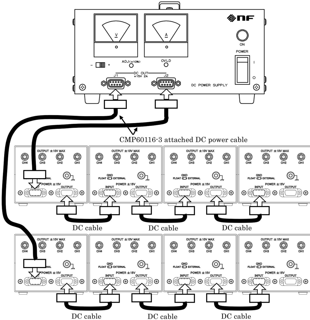
Figure 2-3 Connection when driving 8 products with CMP60116-3.
