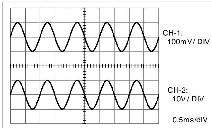
Figure 4-2 Non-inverting input / output voltage waveform.
