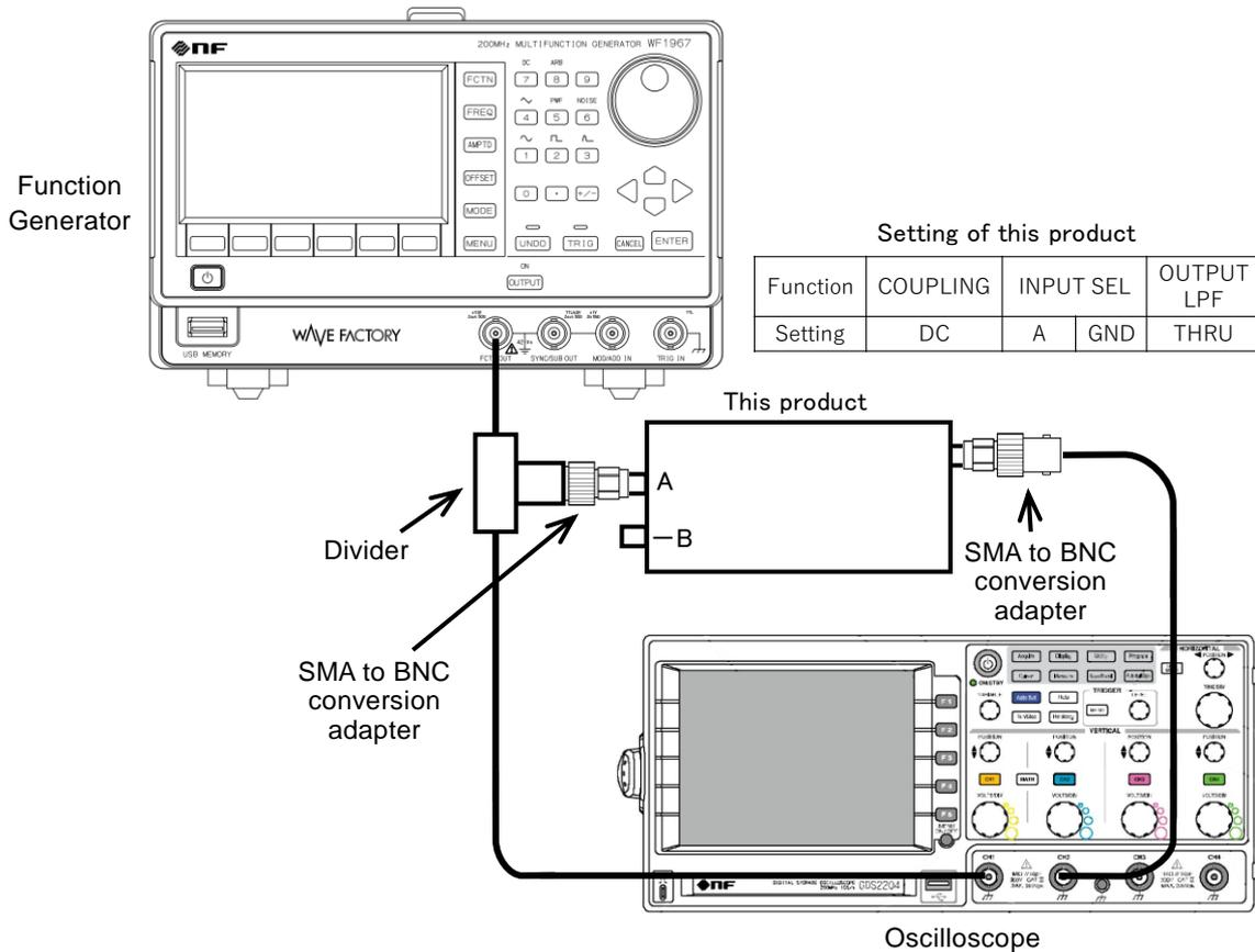
Figure 4-1 Connection diagram for checking non-inverting input operation.
