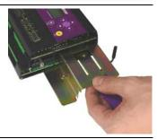
10. Carefully slide the circuit board bundle partially out of the case. Be careful of the flexible cable running between the top circuit board and the keypad. Do not completely remove the circuit boards from the case.
