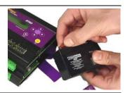
Remove screws on bottom of logger. DT80/81/82 models have two screws, DT85 models have three.
