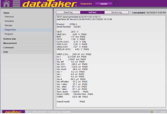
Figure 40: Self Test on Diagnostic screen
