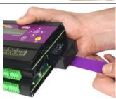
7. Disconnect the battery terminals (models with internal battery only)
