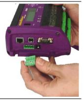
2. Remove the screws from the other end of the logger
