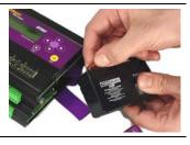
Figure 115: How to remove the main battery
