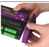
6. Pull the purple 'battery tail' (models with internal battery only)
