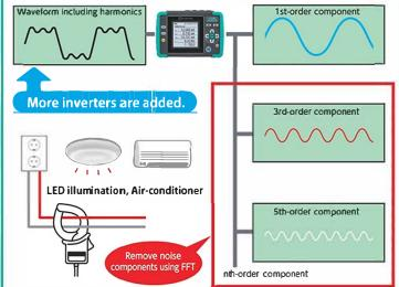
Unlike to traditional for measuring apparatus, less susceptible to harmonics noises, Successfully achieving logging with no effects of harmonics by Trms calculation every 200 ms using FFT (Fast Fourier Transform)
