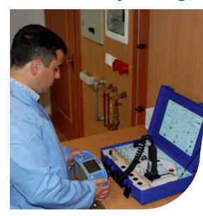
Demonstration board MI 2166 simulates common electrical installation usually met in individual house or apartment. Demonstration board is to be used preferably by sales personnel when demonstrating operation of electrical installation test equipment. Various test methods supported by different test instruments can be presented. MI 2166 is compatible with all Metrel's Installation Safety Testers.
