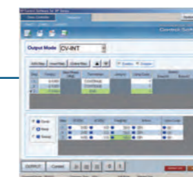
Ex.2 Vehicle Electrical and Electronic Components Test (ISO / DIS7637-2.2 Pulse 4) (Simulation of Transient Voltage Drops at Startup)
