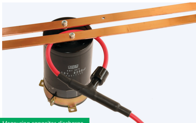
Measuring capacitor discharge
