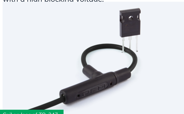
Coil on legs of TO-247
